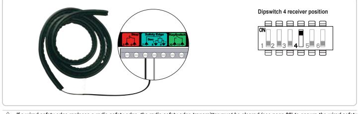
If a wired safety edge replaces a radio safety edge, the radio safety edge transmitter must be cleared (see page 20) to ensure the wired safety edge is taken into account.
