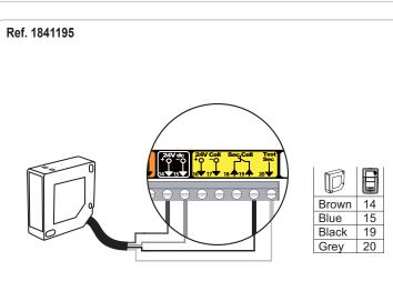
Optical wired safety edge - Dipswitch 4 receiver set at OFF
