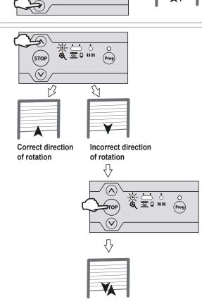
[3]. If the motor end limits are already set, move on to step [8] to exit motor adjustment mode.
