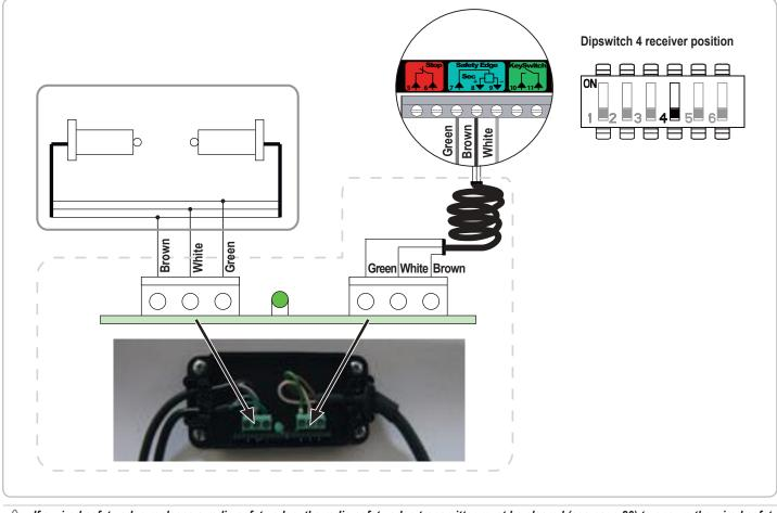
If a wired safety edge replaces a radio safety edge, the radio safety edge transmitter must be cleared (see page 20) to ensure the wired safety edge is taken into account.
