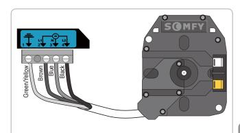
[2]. Lock the motor cable with the cable clamp provided.
