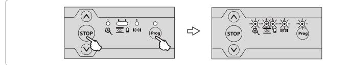
Entry into programming mode by pressing button mode on the receiver is locked.
